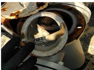
Strainer rupture
